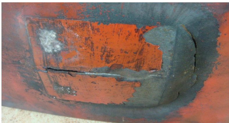
Figure 25 – Large-scale rupture of a steel plate
